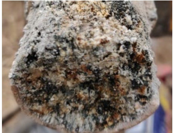
Figure 4-5. Unit 2 Weathered Tonalite
