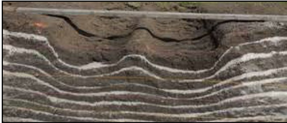
Figure 3-4. Tire Rutting of a Test Subgrade with Low R-Value
